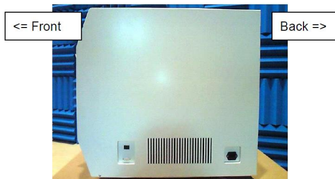
Figure 3. Right-side view of the instrument showing the position of Power Inlet Connector and the Fuse Unit.
