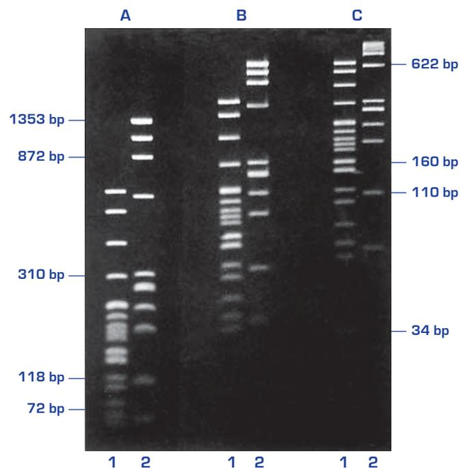
LM SIEVE Agarose gels in 1XTBE buffer A-2%, B-3%, C-4%. Markers: lane 1 - pBR322DNA.MspI; lane 2 - øX174DNA. HaellI. Electrophoresis conditions: submarine gel, 2 hours 30 min., 4.5 V/cm in 1XTBE buffer.
