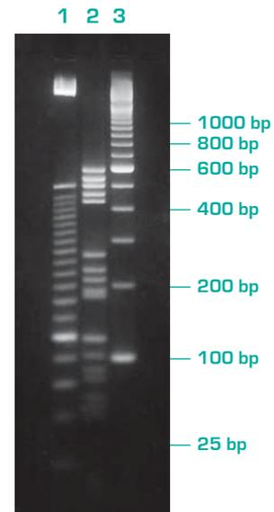
MS-6 3% Agarose gel in 1XTAE buffer. Markers: lane 1 - 25 bp ladder; lane 2 - Molecular weight marker V; lane 3 - 100 bp ladder. Electrophoresis conditions: submarine gel, 2h 30 min, 4.5 V/cm in 1XTAE buffer.
